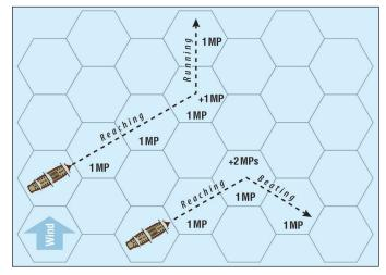
Any other changes in direction do not cost MPs. A ship with only 1 MP (due to rigging damage) may wear in place from Reaching to Running. It may not wear from Reaching to Beating.
